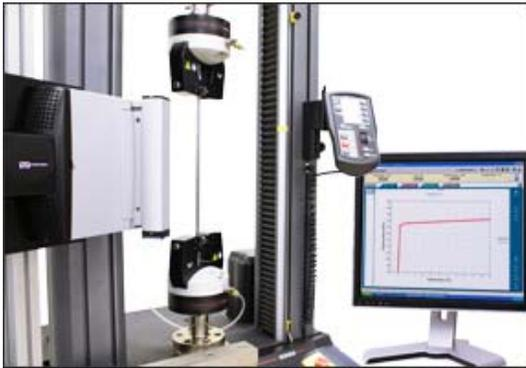
**Q. When testing some specimens, the strain values appear to go backwards when the specimen is yielding. Could extensometer slippage be causing this effect?**
